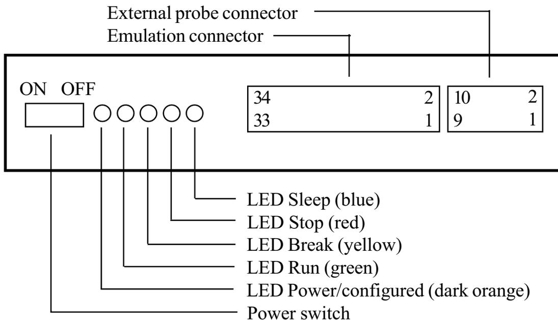
LED Power/configured (dark orange). Blinking / continuous lighting means not configured / configured emulation chip.
